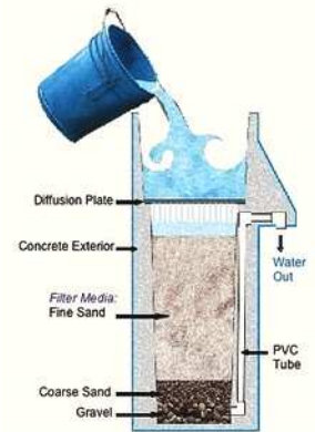
Bio-sand filter in concrete casing
